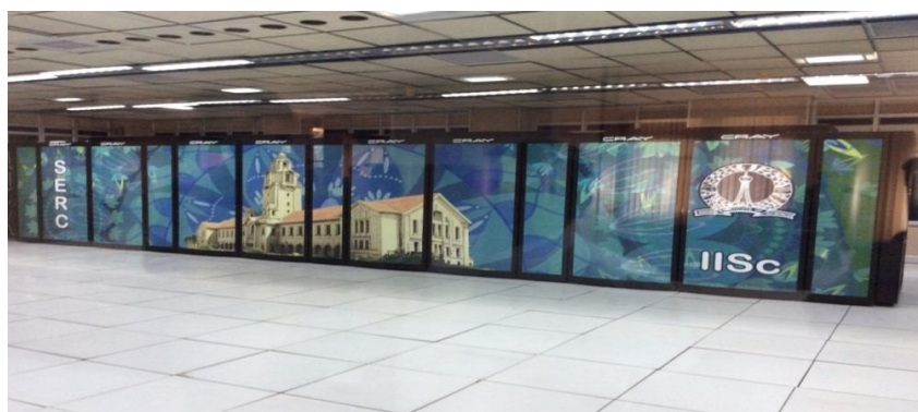
Cray XC40 -India's fastest Supercomputer housed on eight cabinets of 1506 nodes, 1.45PFLOPS and four cabinets of DDN storage with a 2PB usable space 08-01-2016
