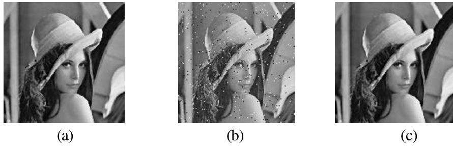
Figure 3.2: Final image obtained after IF median filtering. Figure (a) Input image, (b) Salt and pepper noisy image, (c) Restored image (IF median filtered)
