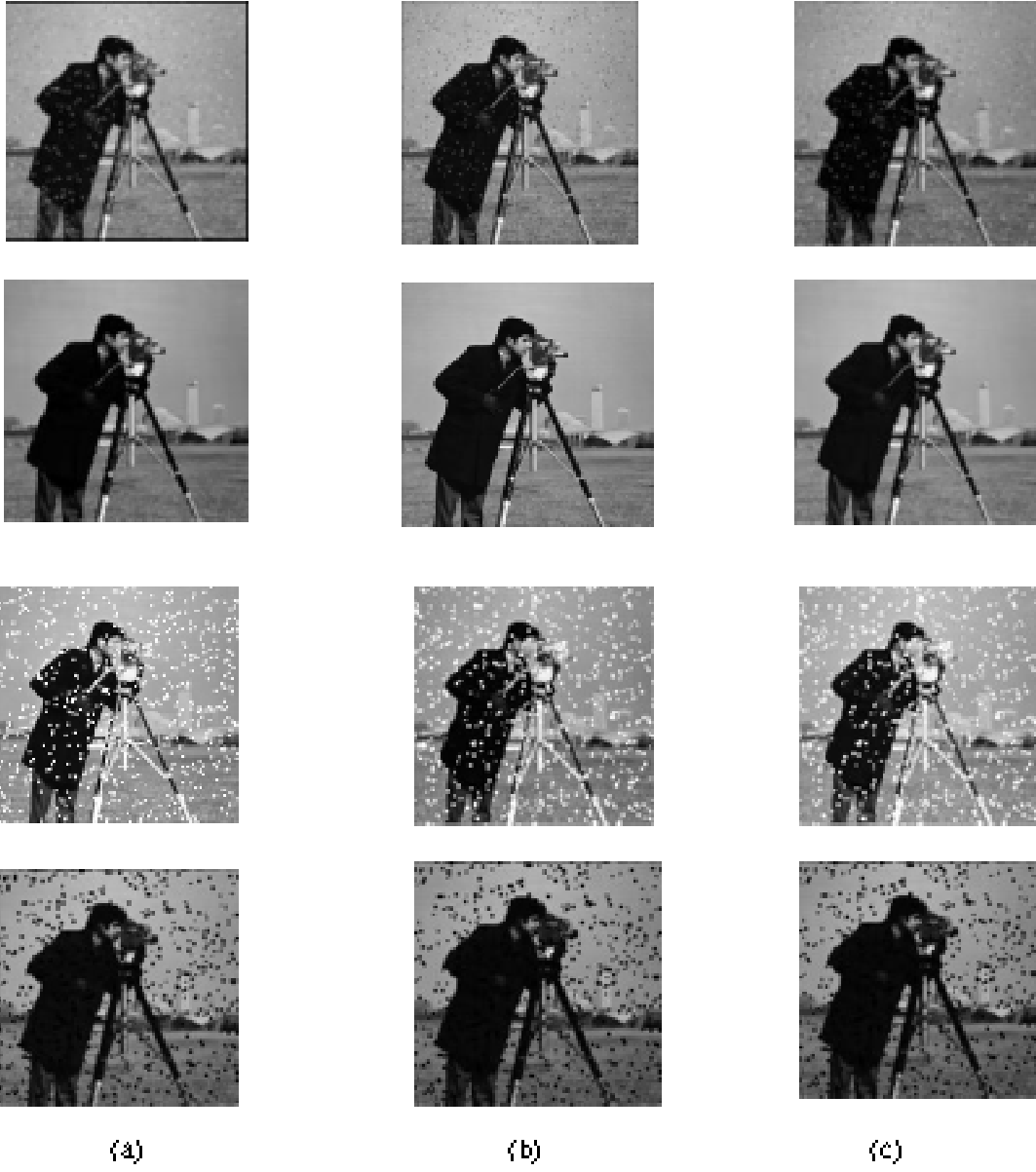
Figure 3.5: Comparison of filters (a) traditional, (b) fuzzy and (c) intuitionistic fuzzy filters.
