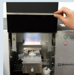
The optimal background correction methods are installed as standard: high-speed self-reversal method (SR method) and deuterium lamp method (D<sub>2</sub> method).
